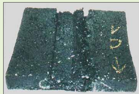
Formation of a rut without EcoStab-7
